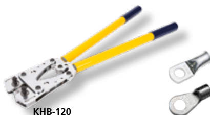
KHB-120 26" Crimping tool for non-insulated terminals 6,0 - 120,0 mm 2 HEXAGONAL crimp
