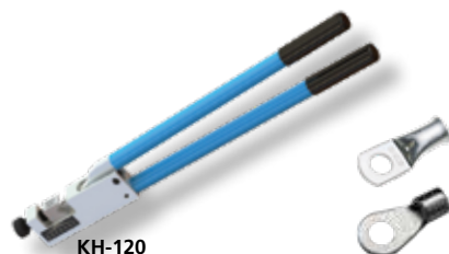
KH-120 26,2" Crimping tool for non-insulated terminals 16,0 - 120,0 mm 2
