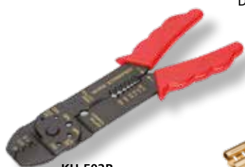
KH-502B 8" Crimping tool for open barrel terminals 0,5 - 6,0 mm 2 Bolt cutting M2,6 / M3 / M3,5 / M4 / M5 Wire stripping 0,75 - 6,0 mm 2
