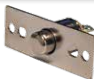
AE-ZZ011 Door contact switch On-(Off) 5A@12V 2 Screw contacts Installation dimension Ø 18,5 mm
