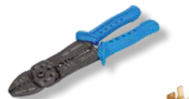
MEB-900C 9" Multi-tool for non-insulated ( brazed seam only ) and open barrel terminals 0,5 - 6,0 mm 2 Bolt cutting M2,6 / M3 / M3,5 / M4 / M5 Wire stripping 0,75 - 6,0 mm 2
