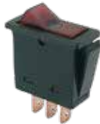
AE-ZZ233 Rocker switch with red LED On-Off 20A@12V 3 Tab contacts 6.3 x 0.8 mm Installation dimension 30 x 12 mm
