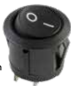
AE-ZZ223 Rocker switch On-Off 16A@12V 2 Tab contacts 4,8 x 0.8 mm Installation dimension 19 x 13 mm
