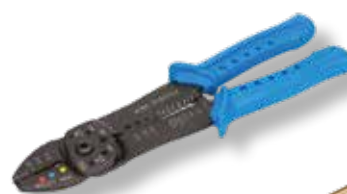
MEB-700C 9" Multi-tool for non-insulated ( brazed seam only ) and open barrel terminals 0,5 - 6,0 mm 2 Bolt cutting M2,6 / M3 / M3,5 / M4 / M5 Wire stripping 0,75 - 6,0 mm 2
