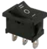
AE-ZZ225 Rocker switch On-Off-On 16A@12V 3 Tab contacts 4,8 mm Installation dimension 19 x 13 mm
