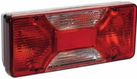
LTL1867 right LTL1852 left LTL1843 lens Iveco Daily Type (new model) Bulbs: 3xP21W, 2xR5W
