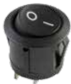
AE-ZZ224 Rocker switch On-Off 16A@12V 2 Tab contacts 4,8 mm Installation dimension Ø 20 mm
