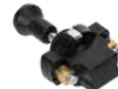
AE-ZZ028 Push-pull switch with small knob On-Off 10A@12V or 2,5A@24V 2 Screw contacts Panel thickness 0,5-2 mm Installation dimension Ø 8,5 mm
