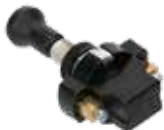
AE-ZZ032 Push-pull switch with small knob On-Off 10A@12V or 5A@24V 2 Screw contacts Length mounting stem 12 mm Installation dimension Ø 8,5 mm
