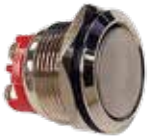
AE-ZZ226 Push button switch On-Off 20A@12V 2 Screw contacts Installation dimension Ø 20 mm
