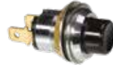
AE-ZZ100 Momentary push button switch (On)-Off 11A@12V or 2,5A@24V 2 Tab contacts Installation dimension Ø 20 mm
