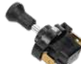
AE-ZZ115 Push-pull switch with small knob On-Off 10A@12V or 5A@24V 2 Tab contacts 6,3 mm Length mounting stem 12 mm Installation dimension Ø 8,5 mm
