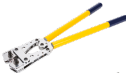
KHB-150 For non-insulated terminals HEXAGONAL crimp 25,0 - 150,0 mm 2
