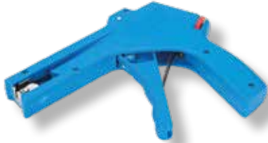
LY-600A For tightening and cutting nylon cable ties 2,4 - 4,8 mm width Thickness up to 1,45 mm Adjustable
