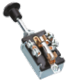
AE-ZZ070 Universal push-pull switch Off-On-On 30A fuse@6V or 15A fuse@12V 5 Screw contacts Length mounting stem 9 mm Installation dimension Ø 11 mm
