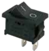
AE-ZZ223 Rocker switch On-Off 16A@12V 2 Tab contacts 4,8 mm Installation dimension 19 x 13 mm
