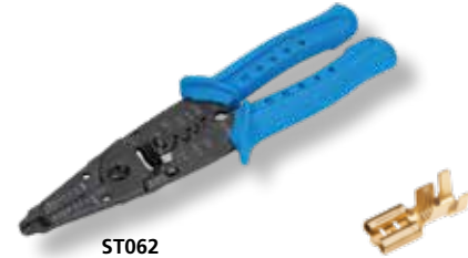
ST062 Multi-tool for Non-insulated ( brazed seam only ) terminals (0,5 - 2,5 mm 2 ), Open barrel terminals (0,25 - 1,5 mm 2 ) and Coaxial cable connectors 6,0 mm Stripping 0,25 - 4,0 mm 2
