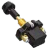
AE-ZZ117 Push-pull switch with small knob On-Off 6A@12V 2 Screw contacts Length mounting stem 13 mm Installation dimension Ø 9 mm
