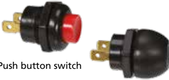
AE-ZZ003 Momentary push button switch with waterproof rubber cover (On)-Off 20A@12V 2 Screw contacts Installation dimension Ø 23 mm
